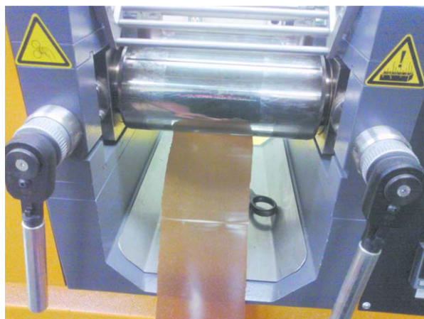
Figure 1. Calendering of MBMPC sheet containing 15 wt % LLDPE using the Collin calender roll. [Color figure can be viewed in the online issue, which is available at wileyonlinelibrary.com .]
